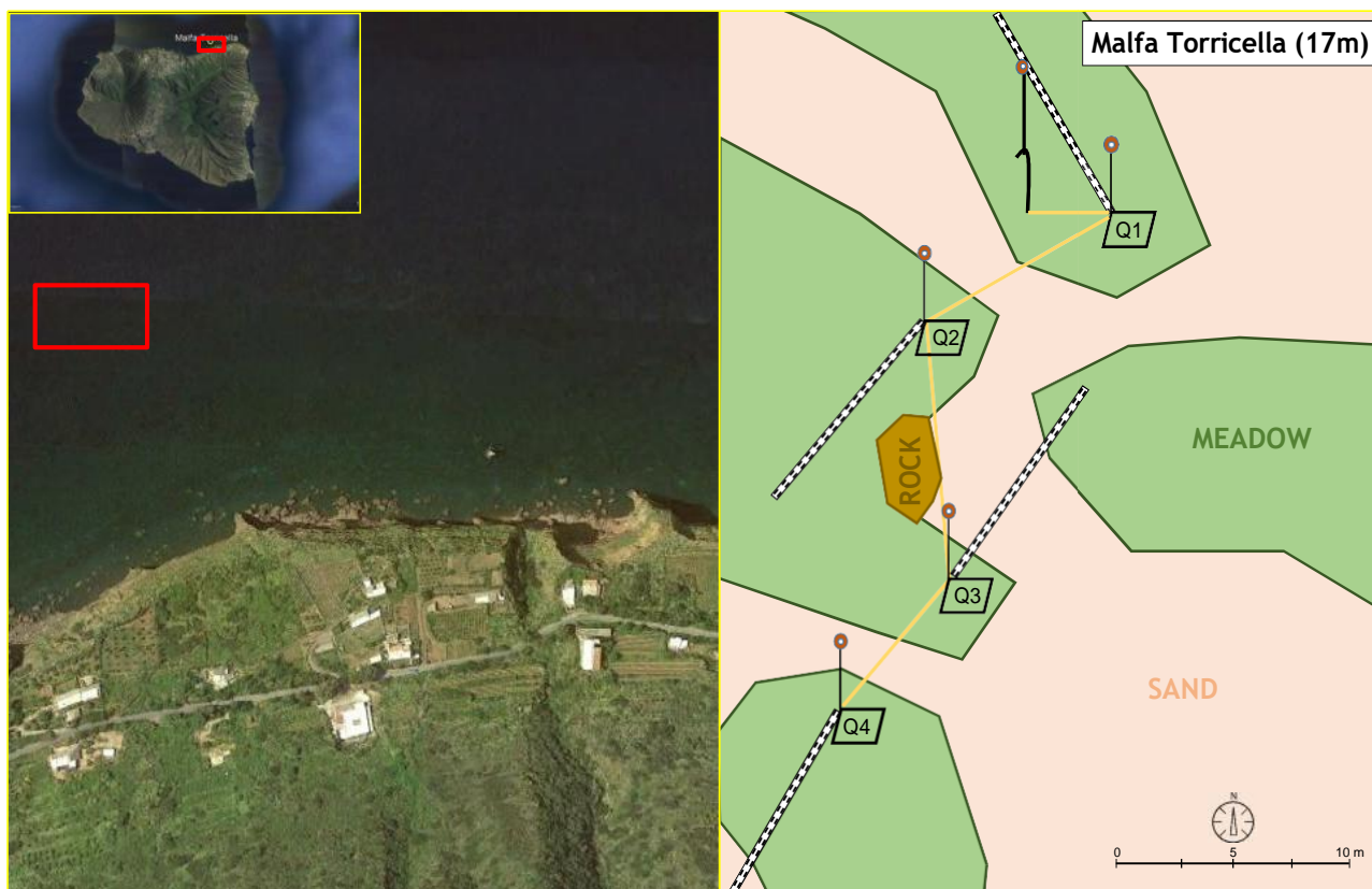
Figure 16. Geographic location of MalfaTorricella station (red square, left panel) and schematic representation of the sampling station with the four fixed 40x40 cm density quadrats (Q1-Q4) and 10-m length cover transects (right panel).
