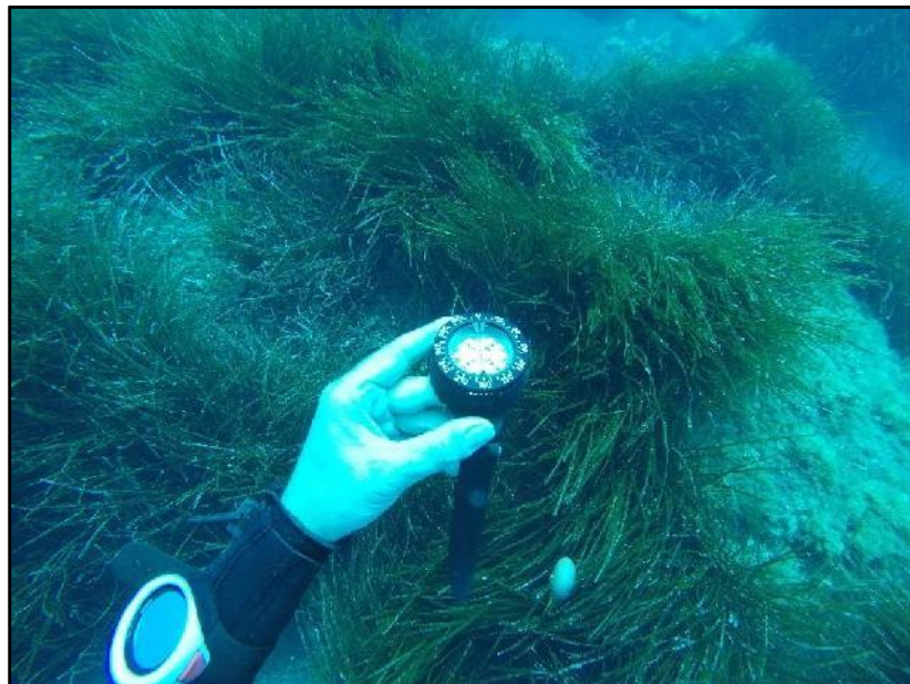
Figure 20. A detailed view of the use of an underwater compass to roll out the 10 meters transect used for the characterization of the meadow cover.
