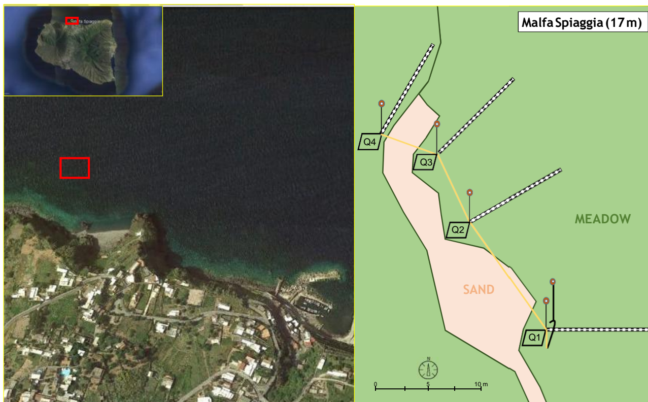
Figure 41. Geographic location of Malfa Spiaggia station (red square, left panel) and schematic representation of the sampling station with the four fixed 40x40 cm density quadrats (Q1-Q4) and 10-m length cover transects (right panel).
